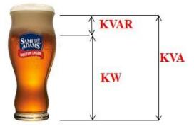
Today, end user facilities are continuing to evaluate solutions and are starting to require that new OEM equipment be compliant with a minimum of 90-95% power factor.
